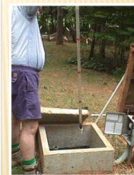
Clear plastic tube with a check valve on the end
